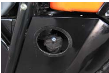
Fuel tank intake (in left side)
